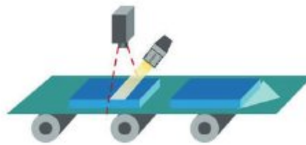
Can be used to detect defects on large-area objects on production lines
