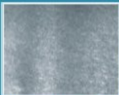
Using standard line light to detect large areas of metal has poor surface uniformity
